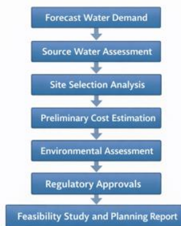
Figure 2: Water Treatment Plant Planning Process Flowchart
