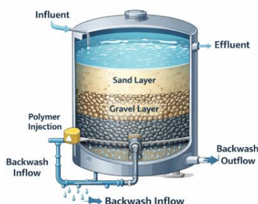
Figure 33: Cross-Section of a Rapid Sand Filter
